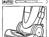
On the AUTO position, the motor power will vary automatically depending on the dirt detected by the dirt sensor
